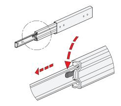
Type F has additionally a detach function through which the extension slides can be completely separated from one another in the area of the middle and inner slide. This feature not only facilitates mounting. It also allows the extension to be quickly removed, for example, when frequent maintenance work is performed on the components located behind.
