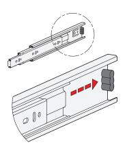
The rubber stops of type F dampen the impact of the slide in the respective end position. This feature minimizes noise development and increases the lifespan. Attached to the slides in a partially concealed, partially visible manner, the stops meet each of the requirements in regard to shape, material, and hardness.
